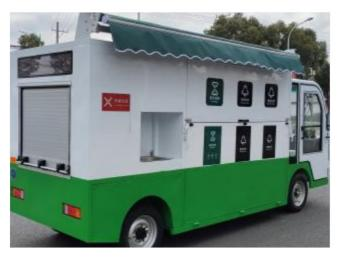
Efficient Operation - 15% gradeability with 7m turning radius
