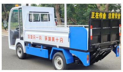
Enhanced Maneuverability - Compact 4.55m length with 6m turning radius
