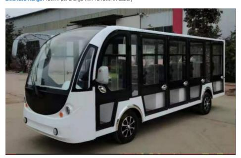
Smooth Operation: 7.5KW motor delivers 35km/h top speed Premium Comfort: Integrated foam seats with leather upholstery All-Terrain Ready: 20% gradeability with 5.5m turning radius
